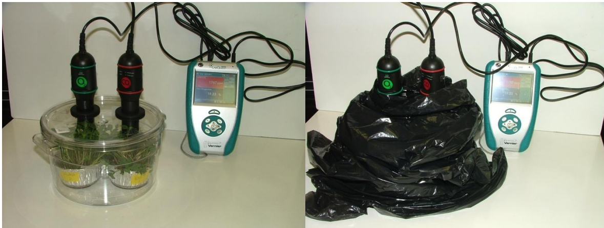
Fig. 2. Illustrating measurement of \text{CO}_2 and \text{O}_2 (optional) concentrations in both light and dark conditions. These measurements were taken in a 2000-mL biochamber available from Vernier Instruments, but could be taken in any reasonably airtight container large enough to hold a number of photosynthesizing plants.
